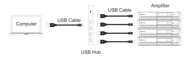
The USB 2.0 standard is restricted to a cable length of 5 meters (15 ft). If you want to control amplifiers over a wider distance, you can use USB range extenders. These extenders boost the USB signal and allow with a LAN cable distances up to 50 meters (150ft) \*). A USB range extender consists of a transmitter and a receiver. The transmitter is connected to the PC on a USB port, while the receiver has one or multiple USB ports to connect the amplifiers.
