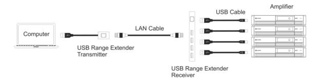
If the amplifiers are placed in different locations (e.g. stage left, stage right), you can use multiple range extenders.
